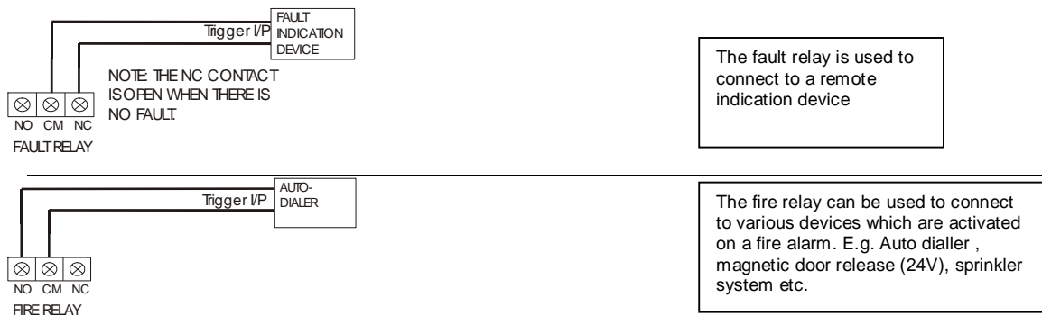
Typical auxiliary output wiring
