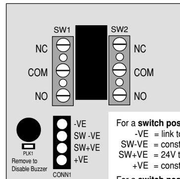
For a **switch positive** trigger connect:-
